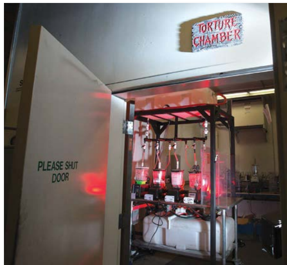
In its "Torture Chamber," Blendtec runs physical tests to see what it takes to break its own products.
