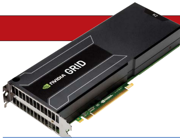
The NVIDIA Grid K2 board, designed to enable multiple users to share a single GPU, is a critical component of the GPU maker’s strategy to capture the virtualization market. Image courtesy of NVIDIA.
